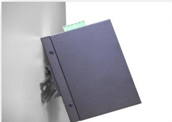
Figure 3.2 - Insert the Switch on the DIN-Rail
